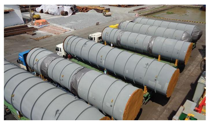
A move of three unassembled air cooling condensers to three different construction sites added layers of complexity to an international logistics solution. Photo credit: Seahawk Logitech.
